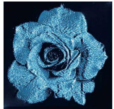
Micro image of "birefringent rose" printed with PHAROS laser in 1 × 1 mm fused silica square. Courtesy of Prof. P. Kazansky, Optoelectronics Research Centre, University of Southampton
