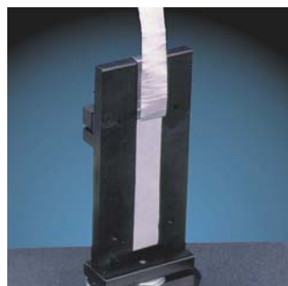
180° Flexible/Rigid Substrate Peel Test
