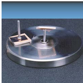
Stud Pull Coating Adherence Test
