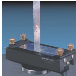
90° Rigid Substrate Peel Test
