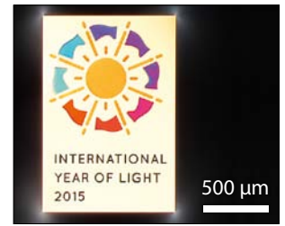
Birefringence modification inside fused silica. Photo in crossed polarized light
