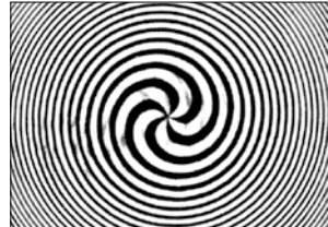
Chrome ablation for beam shaping
