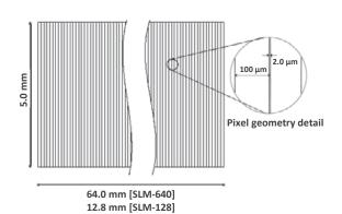
Spatial Light Modulators utilize liquid crystal (LC) masks manufactured in our own stateof-the-art fabrication facility in the U.S. Dual-mask models feature precisely aligned optical masks providing simultaneous phase and amplitude control in a single device.
