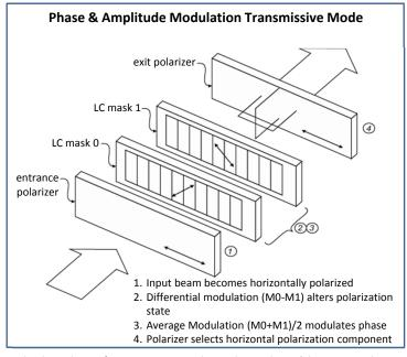
The three choices for transmissive mode are shown above. (The SLM can also be used in reflective mode.)
