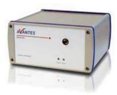
For high sensitivity applications where high resolution is not of paramount concern, the AvaSpec-HS2048XL-EVO is an exceptional instrument. Featuring Avantes' HS optical bench which has a full 0.22 numerical aperture for superior throughput, the AvaSpec-HS2048XL has a backthinned CCD detector with 2048 pixels measuring 14X500 microns.
