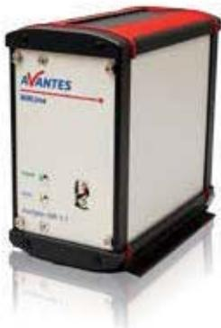
For measurements in the near infrared range out to 1.7 µm, Avantes offers a new series of uncooled spectrometer configurations. The AvaSpec-NIR256-1.7-EVO and the AvaSpec-NIR512-1.7-EVO offer the same high sensitivity optical bench with the next generation of electronics. Both instruments deliver the same exceptional performance specifications such as a sample speed of only 0.53 ms/scan and integration times as fast as 20 µs, as the Avantes instruments you have come to trust.
