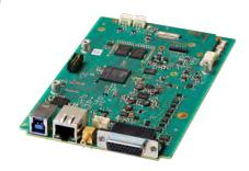
The AS-7010 is the all new electronic platform and the base for Avantes' future spectrometer models.
