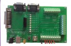
Avantes Spectrometers feature great flexibility offering multiple Input / Output connections. These IO can be used with Avasoft 8 (Time Series) or with customized applications. The DEVKITs are intended to make life easier in the development-stage. Instead of fabricating or soldering a cable with the right connections now it is easy to connect using the screw terminals.
