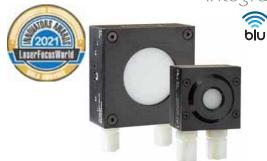
The UP-QED series are power detectors for lasers with extreme power and energy density, such as laser micromachining systems. Thanks to a proprietary absorber that diffuses the measured beam and absorbs it in a larger volume, these detectors have the highest damage thresholds on the market.
