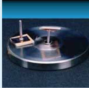
Stud Pull- Coating Adherence Test
