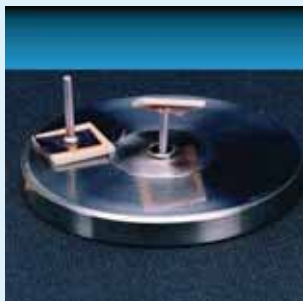
Stud Pull- Coating Adherence Test
