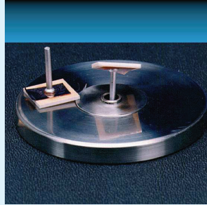
Stud Pull- Coating Adherence Test
