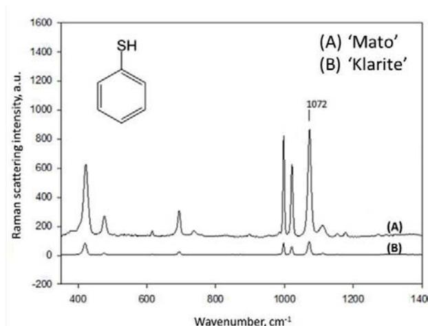
In conclusion, the stochastic nanostructures on soda-lime glass used in 'Mato' SERS substrates, are approximately **8 times** more efficient in comparison to photolithographically etched structures of commercial 'Klarite' substrates
