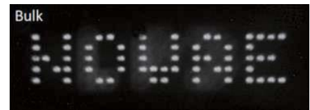
EXAMPLE OF BULK SILICON MACHINING AT 150 \mu m DEPTH
