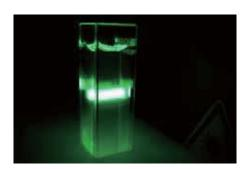
In spectroscopy fluorescence is one of the more challenging setups, due to the low fluorescent emission (about 3% of the excitation energy). The AvaSpec-ULS2048CL-EVO gives the highest sensitivity and the AvaLight-LED series provides excitation at the requested wavelength.
