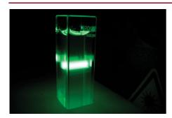
In spectroscopy fluorescence is one of the more challenging setups, due to the low fluorescent emission (about 3% of the excitation energy). The AvaSpec-2048L gives the highest sensitivity and the AvaLight-LED series provides excitation at the requested wavelength.
