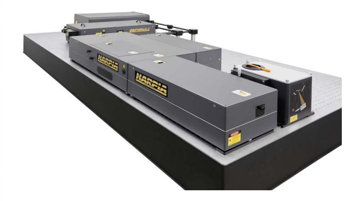
Capabilities of HARPIA-TA spectrometer can be further expanded by HARPIA-TF and HARPIA-TB extensions. Fundamentally, the all-integrated HARPIA system can be viewed as a miniaturized lab facilitating all the most popular time-resolved spectroscopy experiments in a single package. The all-inclusive HARPIA system can provide an extensive comprehension of the intricate photophysical and photochemical properties of the investigated samples.
