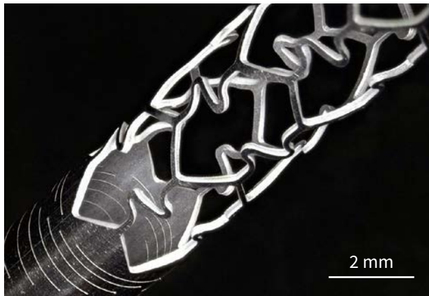
Stent cut using CARBIDE laser. Source: Amada Miyachi America.
