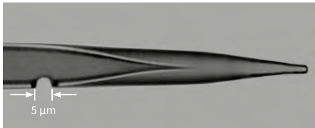
Glass needle microdrilling. Source: Workshop of Photonics.
