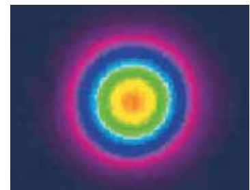
Typical PHAROS far field beam profile at 200 kHz
