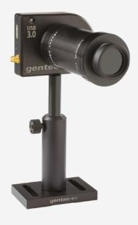
Typically, a CMOS silicon sensor is operating at its full potential when imaging lasers with wavelengths between 350 nm and 1150 nm. If you want to extend the performance range of your Beamage beam profiling camera to the near-IR telecom wavelengths band, you can use the IR Adaptor. This ideal solution takes advantage of a multi-photon absorption process to extend the sensitivity range of the camera sensor to a portion of the near-IR spectrum (1495 nm - 1595 nm).
