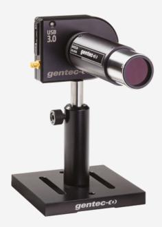
UV Converters take advantage of a phenomenon called fluorescence to extend the performance range of the Beamage beam profiling camera to ultraviolet wavelengths. A fluorescent crystal located at the entrance of the converter absorbs UV wavelengths and reemits longer wavelengths (in the visible spectrum), which are less energetic and detected by the CMOS sensor.
