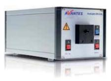
For calibrations in the ultraviolet and visible range (200-1099 nm), the AvaLight-DH-CAL is the best solution. This source can be used with all AvaSpec spectrometers to calibrate for absolute spectral intensity. It is supplied with a built-in diffuser, a cosine corrector (CC-VIS/NIR) with SMA adapter and a CD-ROM containing the calibration
