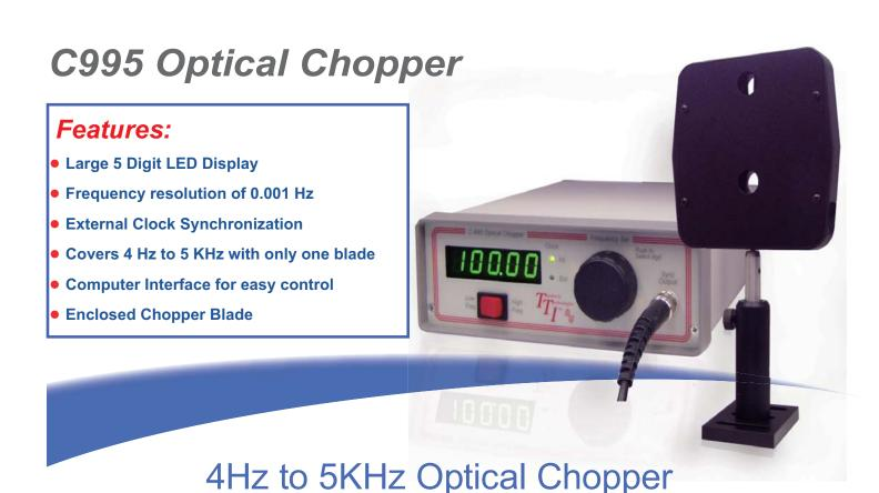
The C-995 is a microprocessor-based control system that utilizes direct-digital-synthesis to deliver precise optical chopping rates from 4 Hz to 5000 Hz. Equipped with a large five-digit LED readout, the C-995 controller enables digital entry of the desired chopping rates from the front panel. Additionally, the C-995 is equipped with a bidirectional Rs-232 port that permits the user to set the desired chopping rate to a resolution of .001 Hz and to read the status of the instrument.
