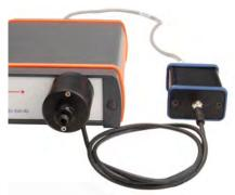
For accurate results during a transmission, absorption, reflection, irradiance or color measurement at different integration times, a good dark measurement is necessary. Taking this dark measurement often leads to having to undertake manual actions, like covering the sensor or switching off the light. This might prove to be problematic with certain applications because of the time and place or operator restraints.
