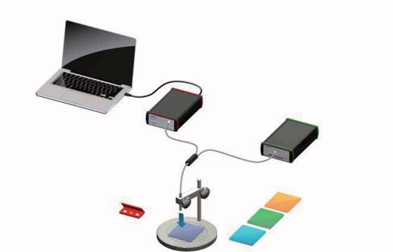
for the software along with characteristics of the thin film layers (material, thickness). Reflectance spectra are captured and analyzed by software algorithms which compare the measured data to theoretical calculated values derived from the database of optical constants. The software provides a calculated thickness value along with a measure of goodness of fit relative to the theoretical curve.
