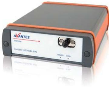
Unique is the second communication port which offers Gigabit Ethernet for integration in your company network and possibility for long distance communication..
