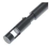
For more flexibility during absorbance measurements in fluids, this fiber-optic probe features a variable and adjustable path length. The gap between the fiber and the diffuser can be set anywhere between 0.25 and 10 mm.
