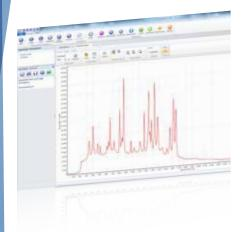
For online and offline reflective color measurements, AvaSoft-COL is the ideal companion. This application provides a precise way to perform color measurements using the basic principles and techniques defined by the International Commission on Illumination (CIE). The CIE 1976 L\*a\*b\* color parameters are calculated, along with other parameters, like Hue, Chroma and X, Y, Z.
