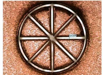
Copper removal from PCB with down to <20 μm resolution.
