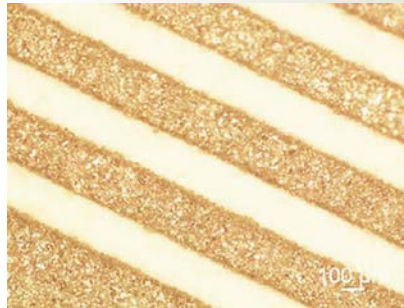
Ablation of 50 μm nickel layer from a ceramic substrate.
