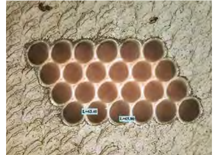
Drilling of 65 μm holes in 0.8 mm PI
