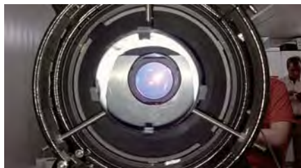
Telescopic optics used in "stand-off LIBS" for an explosives detection several meters away from a sample
