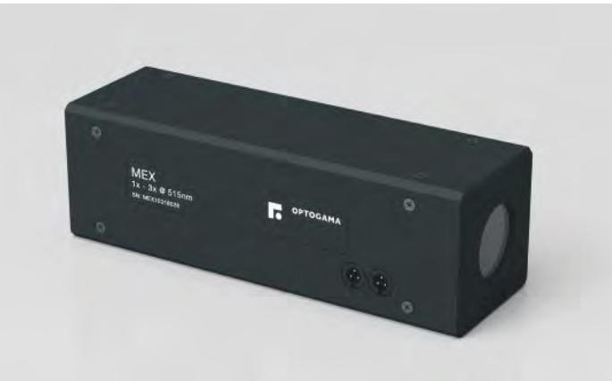
Motorized laser beam expanders MEX series are used to increase the laser beam diameter and adjust divergence. Standard or custom-made beam expanders feature a unique mechanical closed loop sliding-lens design ensuring high pointing stability and minimal dimensions.
