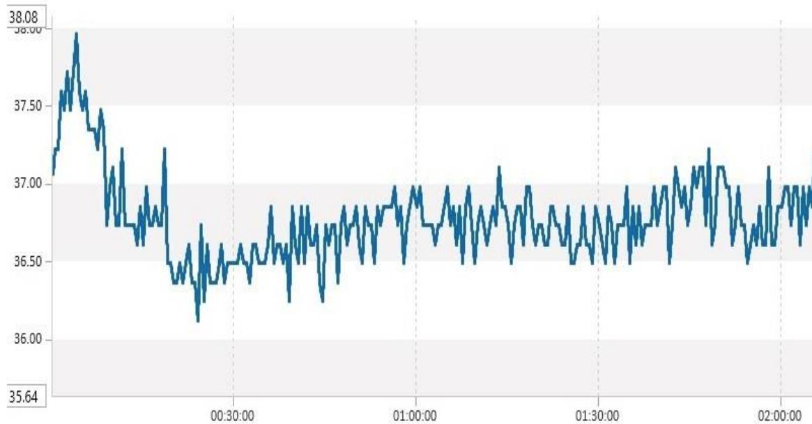
Energy stability measurement of 1kHz laser model. Min. – 36,15 µJ, Max. – 37,97 µJ,
