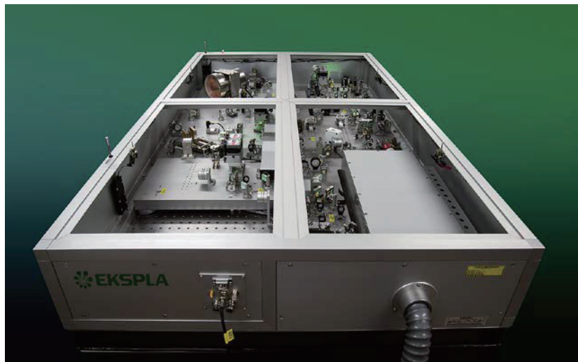
UltraFlux FT310. Customised compact (1.2 × 0.9 m), fully diode pumped, tunable wavelength femtosecond laser system delivering up to 2.5 mJ pulse energy with pulse duration down to 20 fs. Optically synchronized (low jitter) fs and ps outputs available.
