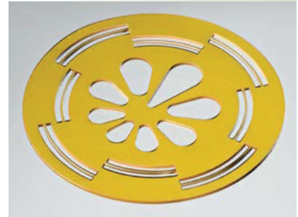
Polyimide cutting. Smallest features down to 165 µm.
