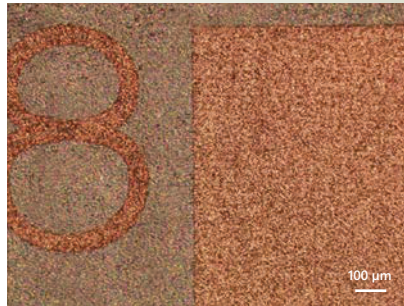
Clear insulation layer removal from flexible PCB. Courtesy of FTMC.
