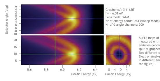
ARPES maps of graphene/Ir(111) sample measured with laser around normal emission geometry showing the Rashbasplit of graphene/Ir(111) surface state. Two different entrance slits of the Electron Analyzer were used, resulting in different energy resolution (marked in the figure).
