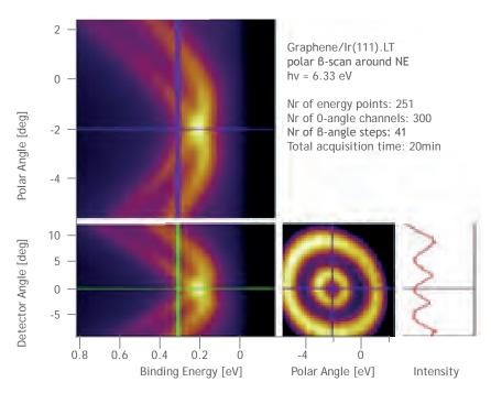
Dependence on Temperature. 3D ARPES data sets for graphene/Ir(111) sample measured with laser (lens mode: WAM). Measurements were performed at T=120K (LT, left) and T=300K RT, right).
