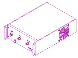
options include a front panel user accessible connection between the oscillator and modulation circuit (N) so that an external source frequency can be used in place of the internal crystal oscillator. Also available is an optional front panel connection between the modulation circuit and the RF power amplifier (H) to give the Model ME drivers capability to be used as a stand alone RF power amplifier. Drivers with option E provide a cw +10 dBm crystal oscillator reference output.
