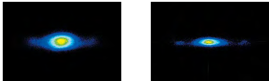
Near field Far field Fig 1. Typical beam profiles of NT242 series lasers at 500 nm
