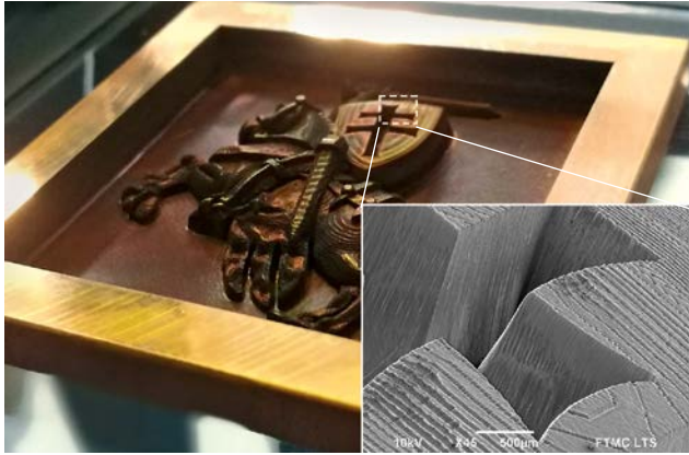
3D milled sample in copper. Zoom in SEM image. Source: “Highly-efficient laser ablation of copper by bursts of ultrashort tuneable (fs-ps) pulses”, A.Žemaitis, P.Gečys, M.Barkauskas, G.Račiukaitis, M.Gedvilas. Scientific Reports (2019).
