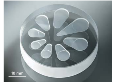
UVFS milling. Courtesy of FTMC.
