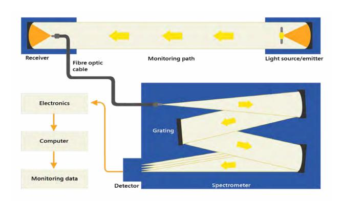
**FIGURE 1**Schematic example of a CEMS using DOAS
