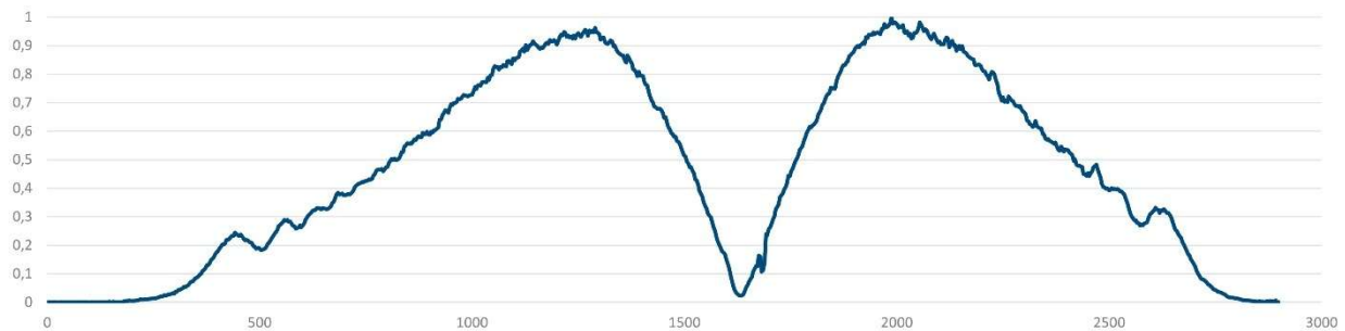
13 fig. Both – positive and negative Bessel beam shaper peak intensity distribution along z – \updownarrow input beam polarization
