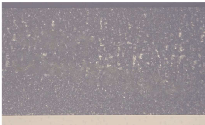
10 fig. Cross-section of glass samples processed using the Beamera Bessel Beam Shaper. Pulse energy: 130 \mu\text{J} on the sample. Pulse duration \sim picoseconds
